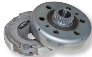
Wet Type Centrifugal Clutch
